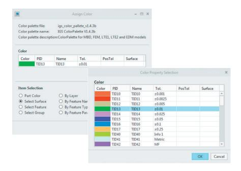
This colour coding system creates different appearance states (i.e. visualisations in the CAD application) for different types of information. One appearance state shows the colours indicating the required tolerances. Each surface area is assigned its own colour, which corresponds with the tolerance given to the surface. A second appearance state displays the assigned surface finishes such as EDM texture or SPI finish.
